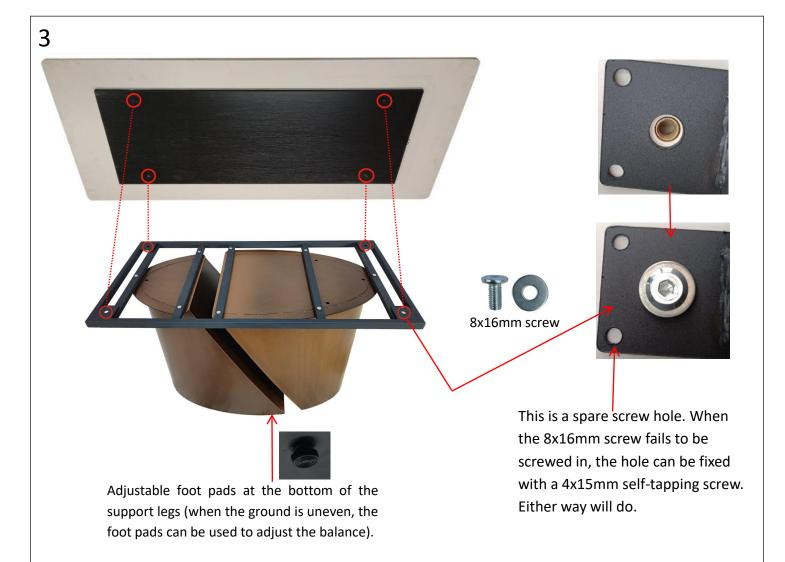
Put the table top on the table leg, make sure the reserved screw holes of the table top and the frame are corresponding, tighten 8x16mm screws from the bottom to finish the installation.
